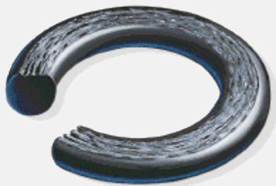
**Description:** The seal or parts of the seal exhibit a flat surface parallel to the direction or motion. Loose particles and scrapes may be found on the seal surface.
