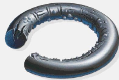
**Description:** The seal exhibits blisters, pits or pocks on its surface. Absorption of gas at high pressure and the subsequent rapid decrease in pressure. The absorbed gas blisters and ruptures the elastomer surface as the pressure is rapidly removed.
