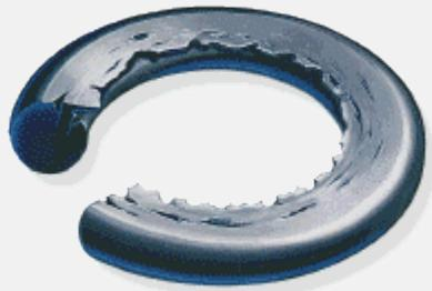
**Description:** The seal develops ragged edges (generally on the low-pressure side) which appear tattered.
