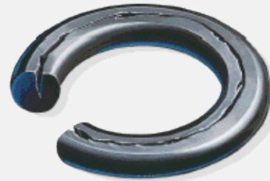
**Description:** The seal exhibits parallel flat surfaces (corresponding to the contact areas) and may develop circumferential splits within the flattened surfaces.
