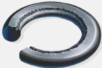
**Description:** The seal often exhibits discoloration, as well as powdered residue on the surface and possible erosion of elastomer in the exposed areas.
