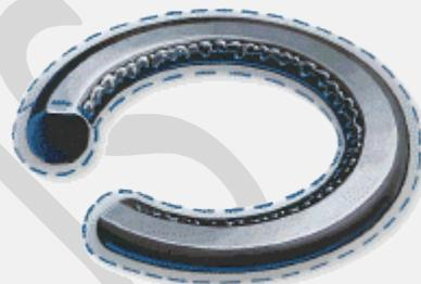
**Description:** This failure is often very difficult to detect from examination of the seal. The seal may exhibit a decrease in cross-sectional size.
